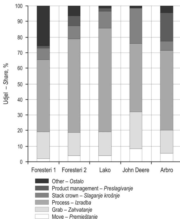
**Fig. 2** Breakdown of net cycle time
