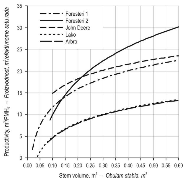
**Fig. 1** Net productivity as a function of stem volume, for the different tests
