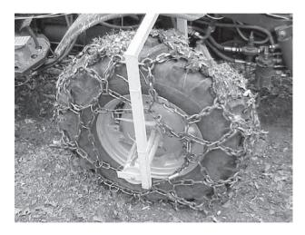
Fig. 7 Chains on a tractor drive wheel
