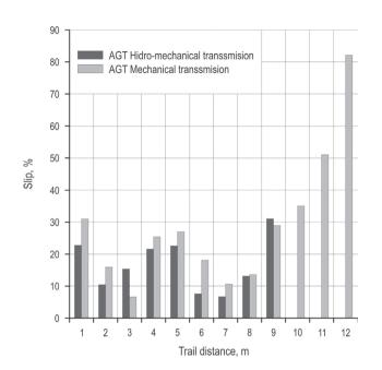
Fig. 12 Comparison of wheel slip between tractors
