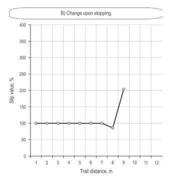
was marked as level 100). This value was compared with the values in the last two meters of load skidding. An approximately twofold increase in the slip value was recorded in the last meter of movement (Fig. 10B). At this point the tractor stopped.
