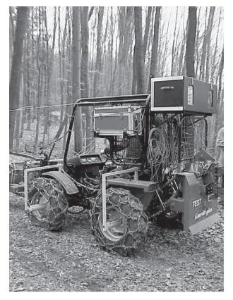
Fig. 2 Adapted agricultural tractor AGT 835 T with measurement equipment
