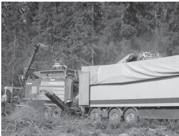
**Fig. 2** Integrated grinding and screening of stumps for fuel at the roadside landing (ground stump wood was discharged into a walking floor semitrailer via a conveyer belt, and screening reject was removed back to the landing area via a side conveyer belt)
