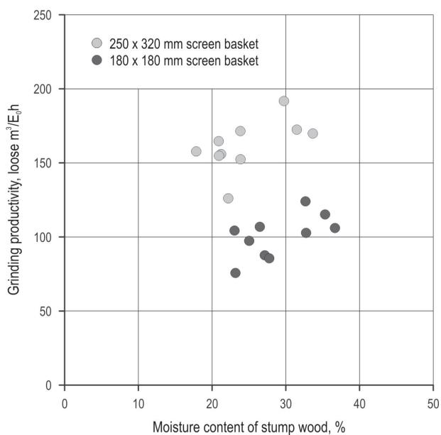
**Fig. 5** Grinding productivity according to moisture content of stump wood (%), for the two screen baskets considered
