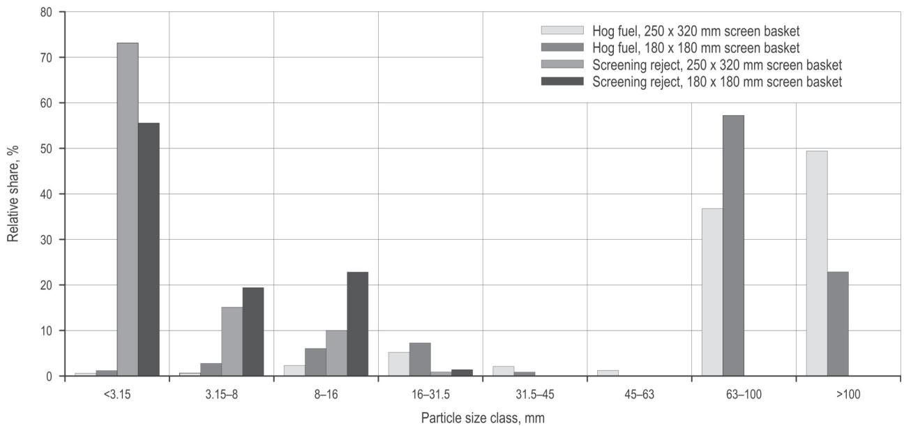
Fig. 8 Particle size distribution of screening reject and hog fuel when using the 250 x 320 mm and 180 x 180 mm screen baskets
