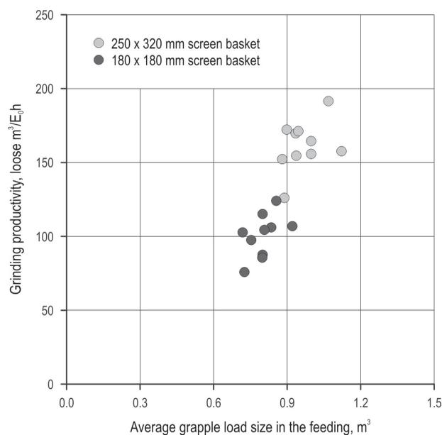
**Fig. 4** Grinding productivity according to load size in the feeding, for the two screen baskets considered
