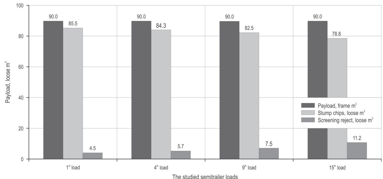
**Fig. 6** The volume of screening reject per studied semitrailer load (a screen basket of 250 x 320 mm was used for loads 1, 4, and 9, and 180 x 180 mm for load 15)
