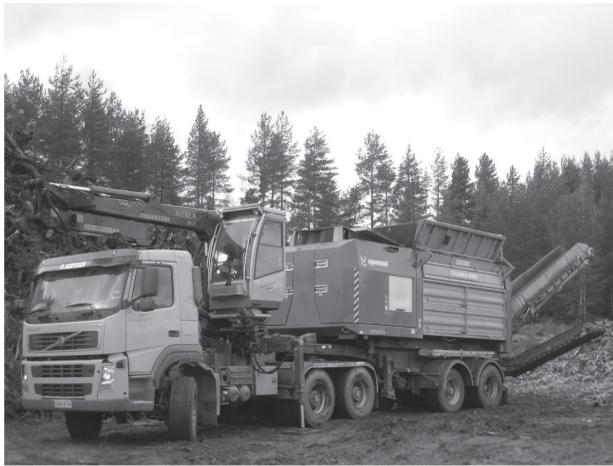
**Fig. 1** The tandem-axle semitrailer-mounted Crambo 6000 low-speed double-shaft grinder equipped with a star screen and heavy-duty Kesla 2012T cab timber loader
