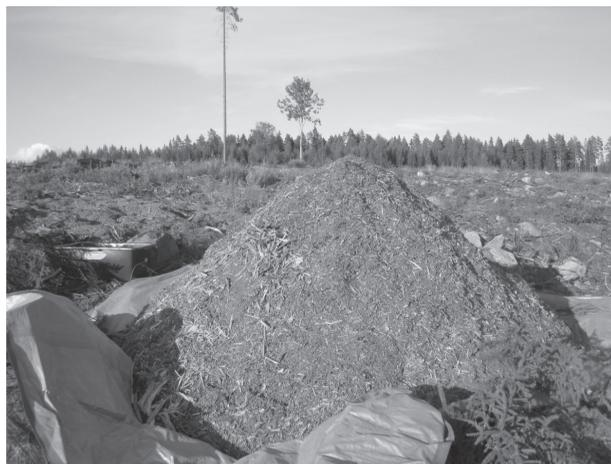
**Fig. 3** A mound of screening reject from the first semitrailer load, on a tarpaulin, after integrated screening and grinding of stumps at a roadside landing
