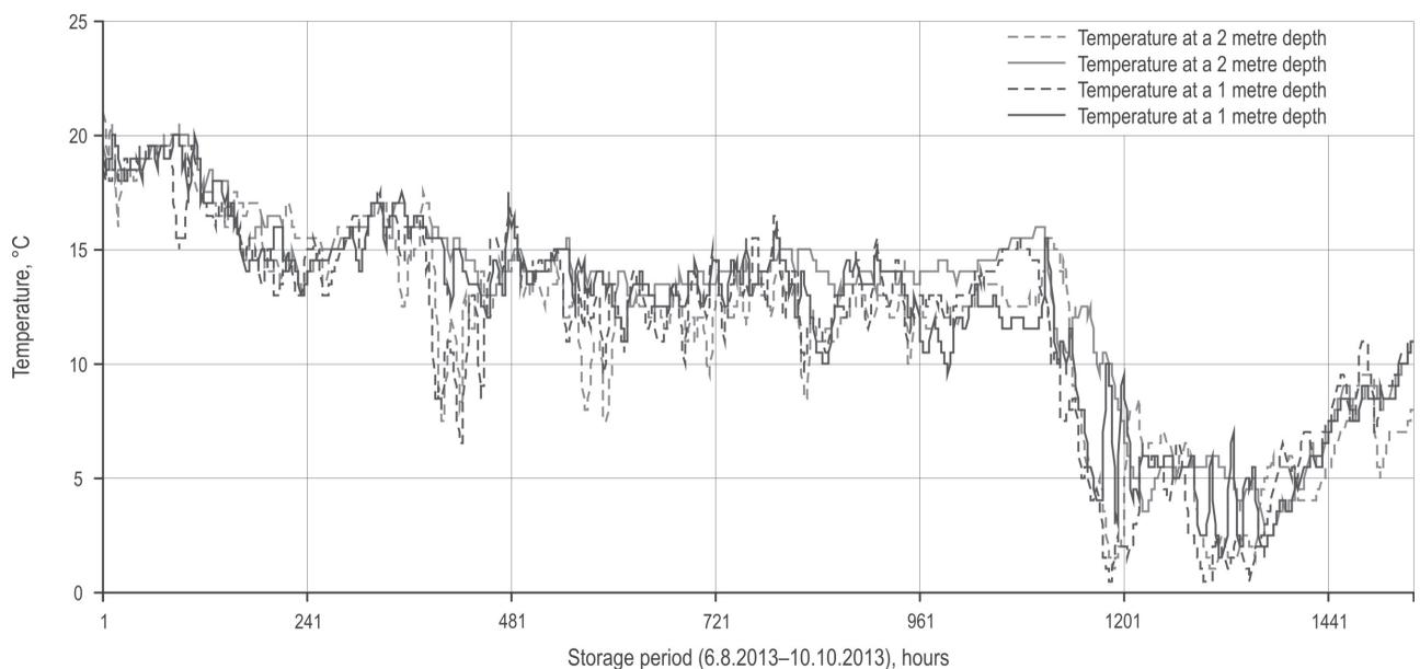
Fig. 9 Temperatures of ground stump wood (hog fuel) at a terminal stack at 1 and 2 meter depth
