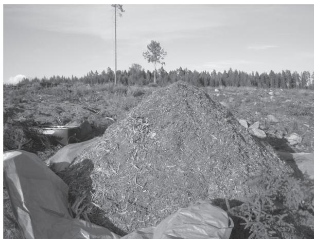
**Fig. 3** A mound of screening reject from the first semitrailer load, on a tarpaulin, after integrated screening and grinding of stumps at a roadside landing
