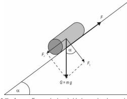
Fig. 3 The forces affecting the log skidded on inclined ground *Slika 3.* Utjecajne sile pri vuči trupca na nagibu
