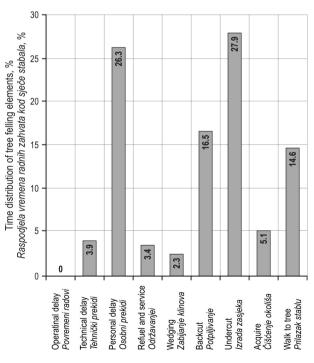
**Fig. 9** Percentage of time distribution of tree felling elements *Slika 9.* Postotna distribucija vremena radnih zahvata prilikom sječe stabala
