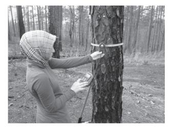
**Fig. 3** Light conditions being measured using the Mastech LX1330B light meter
