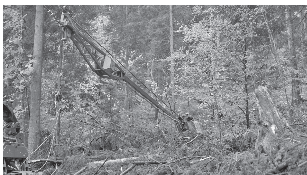
Fig. 4 Contractor-developed double-hitch carriage (here: not in use) (image credit: Schweier/WSL)
