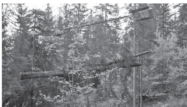
Fig. 5 Double-hitch carriage in use. The end of the tree/piece shown uphill/right is attached to the carriage we call »carriage 1«, while the end of the tree/piece shown downhill/left is attached to what we call »carriage 2« (image credit: Schweier/WSL)
