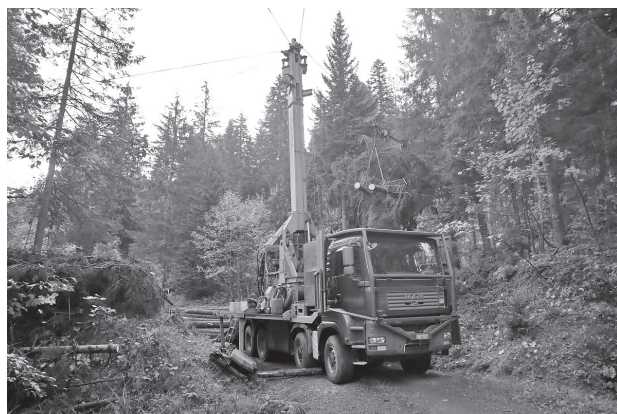
Fig. 3 Koller tower yarder with a mounted processor installed on a truck (image credit: Schweier/WSL)
