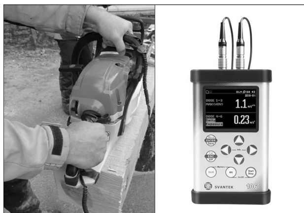
Fig. 2 Six-channels human vibration meter Svantek mod. 106
