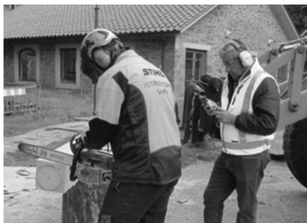
Fig. 5 Vibration measurements during cross-cutting
